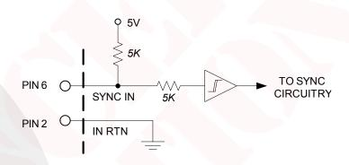
Figure B: Equivalent circuit looking into the SYNC IN pin with respect to the IN RTN (input return) pin.
