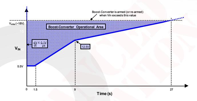
Under-Voltage Transient Profile showing when the boost-converter is guaranteed to be operational. Before the boost converter will operate, it must first be armed (or re-armed) by making  $V_{IN}$  greater than  $V_{ARM}$ .
